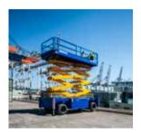
The HL-275 is the first of a new range of hybrid powered scissor lifts from Holland Lift, and the first ever to use a parallel hybrid system.
