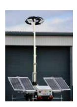
The SMC Solar is a lighting tower without a diesel engine, powered by solar panels and battery pack, meaning no fuel, no engine oil, zero noise and zero CO2 emissions. Run time is indefinite with peak solar conditions, with mains charging of batteries also an option.
