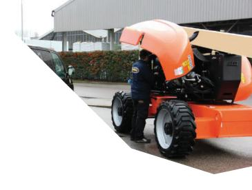
Advances in telematics also permit the device to communicate with the access platform's CAN Bus system, which provides remote access to diagnostic fault codes.
