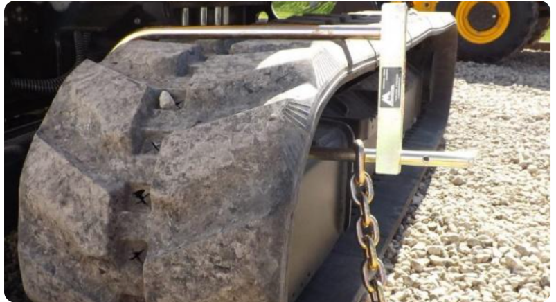
Heavy-duty track lock — prevents movement and theft of small tracked machines
