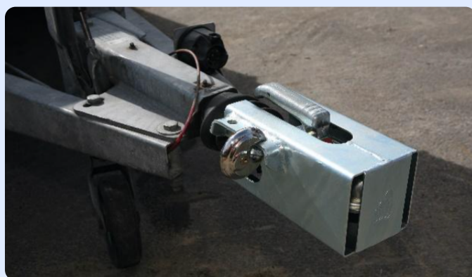
Trailer hitch lock — prevents unauthorised towing and theft.
