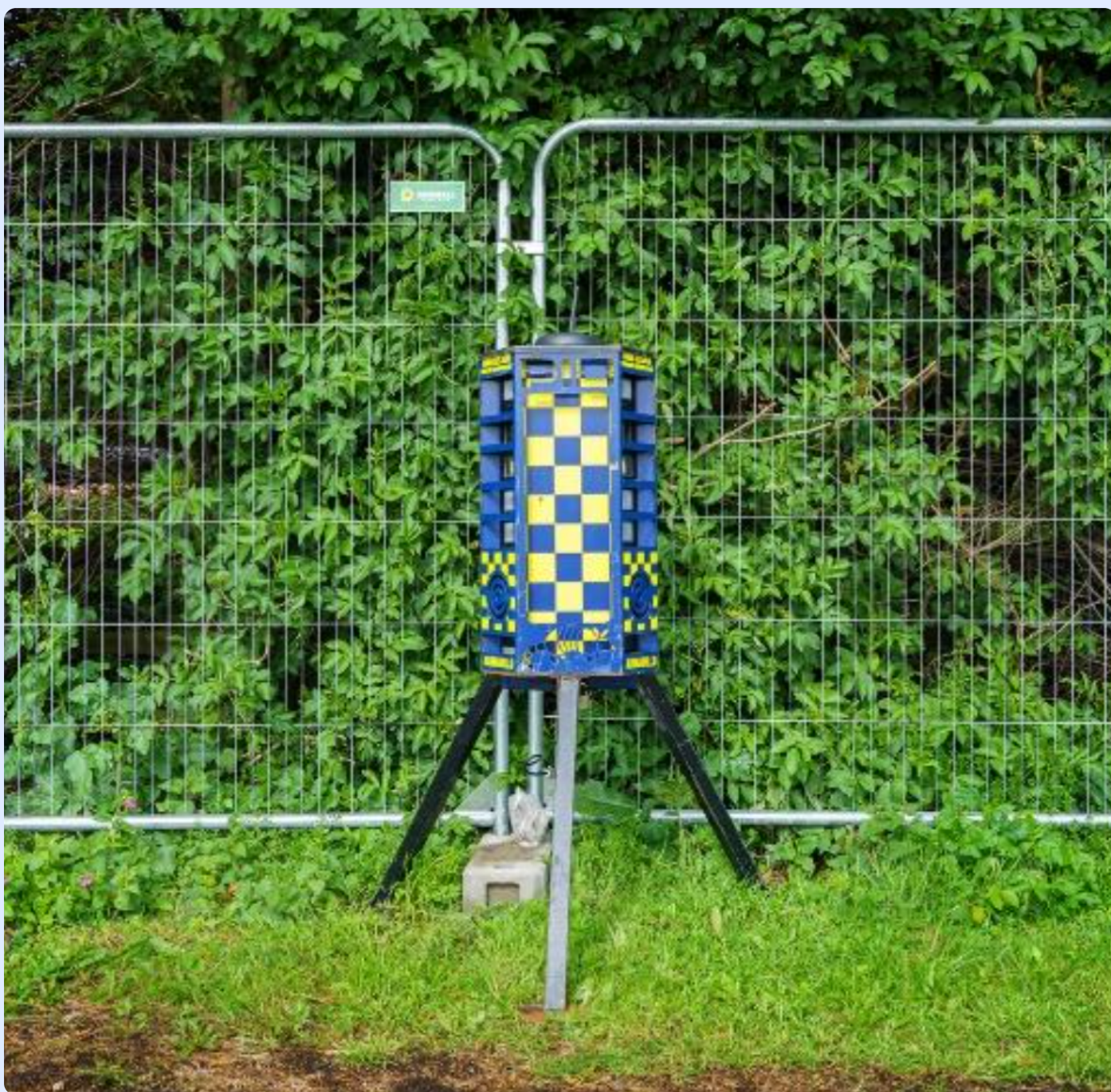
Perimeter intrusion detection system – monitors site boundaries and alerts to unauthorised access.
