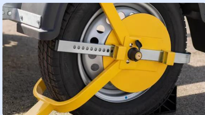
Use a wheel clamp to prevent theft and unauthorised movement.
